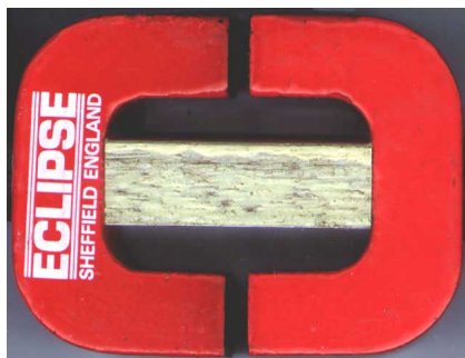
Figure 25 Two C Magnets with wood spacer.
