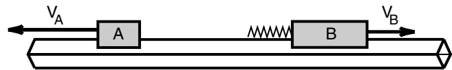
Figure 3 Definition of mass. When two carts recoil from rest, the more massive cart recoils more slowly. (See Figure 6-3)
